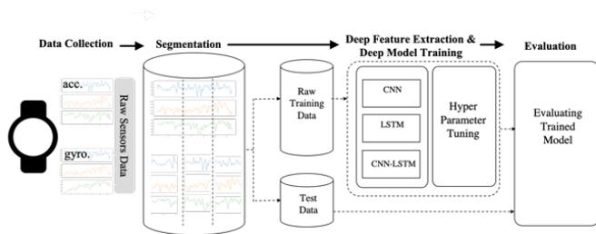
Fig. 1. The proposed framework of smartwatch-based HAR
