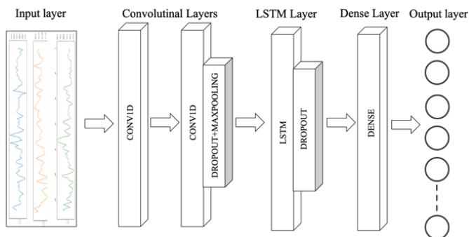
Fig. 2. The structure of the proposed CNN-LSTM network
